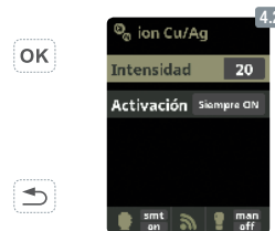
4.2 Intensity in mA: Recommended value within 20 to 50 mA. Recommended timer setting: Pr 10
