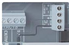
Free Chlorine probe ③ red ④ black
